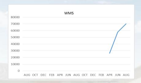
The WMS chart has been reconfigured to include the following 7 meters: 755 park high and low flow, BO and Team High, Pit house, buss barn, athletic field and DO. All of these meters are totaled on the WMS graph but each data point is recorded separately to aid in identifying leaks. A large leak was found on the irrigation line on the Park street meter responsible for the large spike in AUG, balance of spike from April is due to irrigation.
